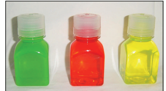
REC coolants: Conventional, Extended Life, and Hybrid.
